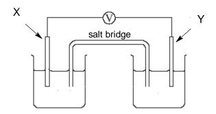
Which of the following combination of metals would produce the highest reading on the voltmeter?
