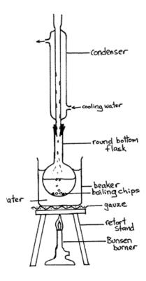
Retort stand, clamps and bossheads have not been drawn for clarity of diagram Flask should have alkanol, alkanoic acid, conc.  $H_2SO_4$
