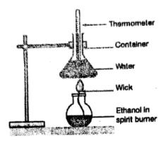
$100.0 \,\mathrm{mL}$  of water at  $298 \,\mathrm{K}$  was heated by the burning of  $1.20 \,\mathrm{g}$  of ethanol in the spirit burner. Only  $45.0 \,\%$  of the energy produced is used to heat the water. The molar heat of combustion of ethanol is  $1368 \,\mathrm{kJ} \,\mathrm{mol}^{-1}$ . Calculate the final temperature of the water.
