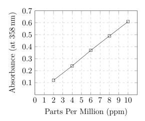
(b) The water sample collected provided an absorbance reading of 0.54. The Australian Drinking Water guidelines state that the safe limit for chromium(VI) is 5 mg/L. Use your graph to determine whether the water sample tested was fit for consumption.
