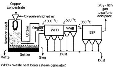
ESP = electrostatic precipitator
