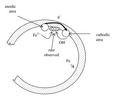
Identify the oxidation state of iron in the rust observed on the inside of the pipe.
