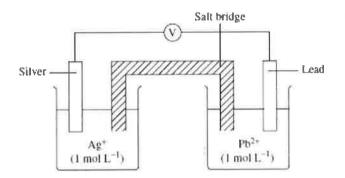
(a) On the diagram, clearly identify the anode and the direction of electron flow in this cell.
