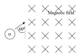
The velocity of the alpha particle is  $2 \times 10^3$  ms<sup>-1</sup>, the charge on the alpha particle is  $3.2 \times 10^{-19}$  C, and the strength of the magnetic field is 0.5T. The magnitude of the force on the alpha particle is then:
