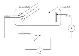
In experiments using this apparatus to determine the work function of different materials, photoelectrons are stopped from reaching the collector.
