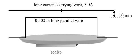
The conductors are parallel for 0.500 m, and are separated by 1.0 mm. A current of 5.0 A is flowing through the top conductor. When a current flows through the conductor, which is resting on the scales, the scales measurement *decreases* by  $4.50 \times 10^{-4}$  kg.
