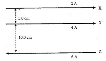
Calculate the magnitude AND direction of the force per unit length on wire Y, due to the other two wires.
