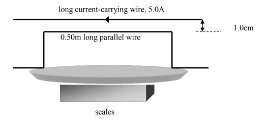
The conductors are parallel for 0.50m, and are separated by 1.0cm. A current of 5.0A is flowing through the top conductor. When a current flows through the conductor which is resting on the scales, the scales measurement *increases* by  $3.50 \times 10^{-4}$ N.
