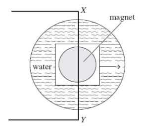
When the current was passed through the wire the magnet moved to the right, as shown by the arrow.
