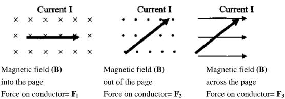
Which of the following correctly compares the magnitude of the forces FI, F2 and F3?
