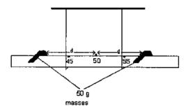
The ruler was set oscillating so that it swings in a horizontal plane. The period, T, of oscillation was determined experimentally for various values of the distance, d, the distance of each mass from the centre of the ruler. The table in your Option Answer Booklet Two records the period, T, and the distance, d for different values of d.
