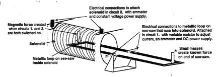
The see-saw is initially balanced. A small mass was placed at the end of the see-saw outside the solenoid to create a known force. With both circuits on, the current flowing into circuit 1 was adjusted till the magnetic force on the see-saw, created on the current carrying metallic loop inside the solenoid, balanced the force created by the mass at the other end. The current through the solenoid in circuit 2 remained constant throughout the experiment. The following data was collected:
