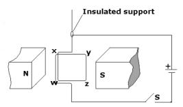
Which of the following statements describes the response of the coil when the switch S connecting the coil to a DC voltage supply is closed?
