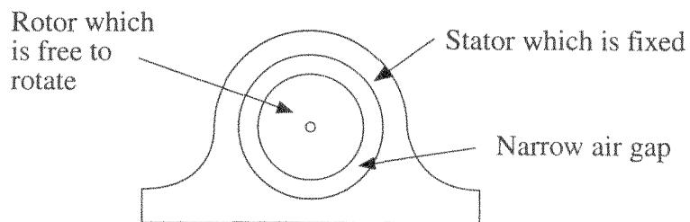
When connected to an ac supply, the stator generates a magnetic field ( $B$ ) that rotates the air gap with constant speed ( $v$ ).
