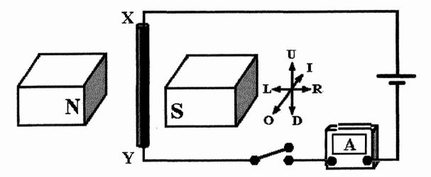
A perpendicular axis system is shown in the diagram, labelled: up (U), down (D), left (L), right (R), into page (I) and out of page (O). The conductor is free to move in any of these directions.
