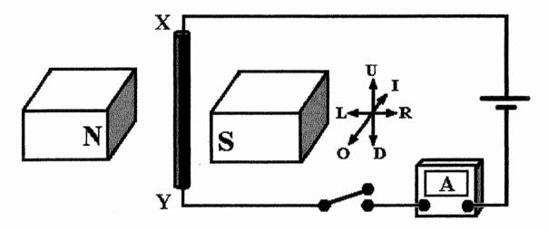
A perpendicular axis system is shown in the diagram, labelled: up (U), down (D), left (L), right (R), into page (I) and out of page (O). The conductor is free to move in any of these directions.
