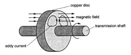
There is a magnetic field through part of the disc when slowing the vehicle. As the copper disc rotates, eddy currents apply a braking force to the shaft.
