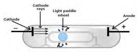
Connection to high voltage sparking coils to produce discharge but do not turn on till certain all is correct.. Ensure the direction of the "positive" and "negative flow of current is known so that the cathoide is identified. Ensure the setup is perfectly level on a flat surface. Ensure all safety precautions are in place so that electric shocks do not occur.
