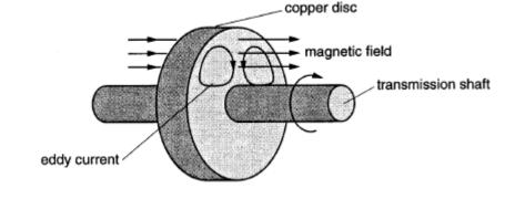
There is a magnetic field through part of the disc when slowing the vehicle. As the copper disc rotates, eddy currents apply a braking force to the shaft.
