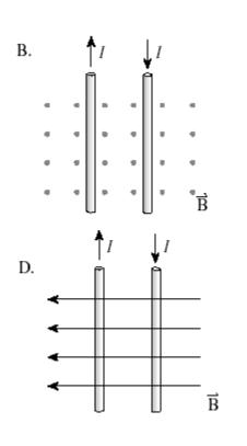
8. An electron, travelling with a constant velocity, enters a region of uniform magnetic field, B. Which of the following is **not** a possible pathway? **D**
