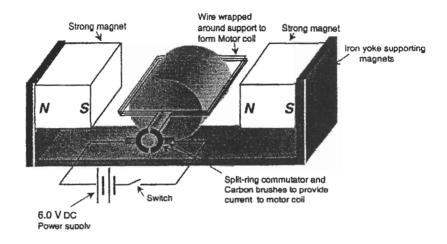
The student conducted tests on the motor and found that it operated best when using a 6.0 volt power supply, with the motor rotating at a frequency of 3 hertz.
