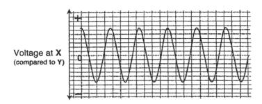
Considering the graph starts with the generators in the positions shown, which of the following alternatives would correctly represent the direction of rotation and form of generator that produced the plot shown.
