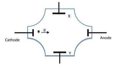
(a) Describe and explain the path taken by q if a voltage of 24 000 V is put across XY, with X being positive.
