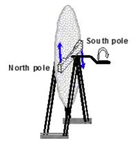
The device shown in this diagram is called an Aragó disc. The actual disc is a circular plate made of aluminium or copper, which can rotate freely on a crank handle. There is a long horseshoe magnet attached to the crank handle, so when it is turned the poles of the magnet move across the surface of the plate, which is observed to rotate in the same direction as the magnet is moving.
