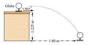
A frictionless glider is moving at a uniform speed  $v \text{ m s}^{-1}$  across a smooth horizontal table 1.225 m high when it reaches the edge, and falls to the floor and lands 1.8 m away from the table.
