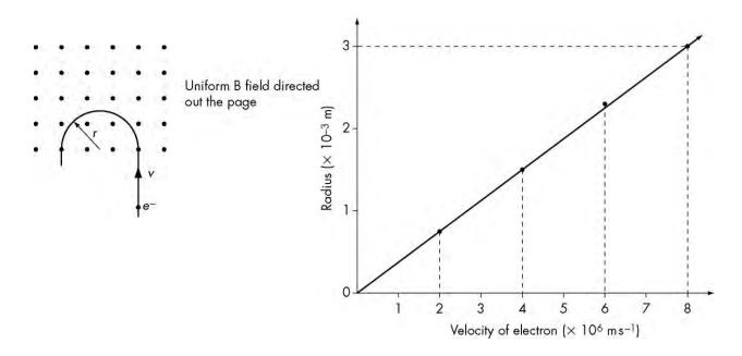
(a) By equating the centripetal force and magnetic force on a charge moving at right angles to a magnetic field at a constant speed (v) derive a general expression for the radius of curvature of the charge in the field.
