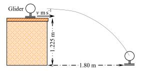
A frictionless glider is moving at a uniform speed  $v \text{ m s}^{-1}$  across a smooth horizontal table 1.225 m high when it reaches the edge, and falls to the floor and lands 1.8 m away from the table.
