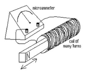
Another acceptable answer would be to draw and label a generator, and explain how the rotating coil undergoes a change in mag flux to generate PD (and a current if in a complete circuit).
