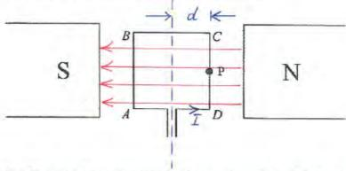
When the coil is connected to an external circuit and a current is passed through it, the coil—though wanting to rotate—is held stationary by a 5.0 g mass (attached at point P; the weight force of the mass is directed INTO the page).
