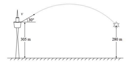
(a) Calculate the horizontal distance away from the tower that the fireworks explode
