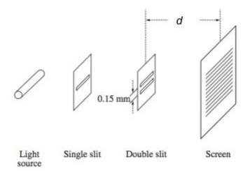
If the distance between the central bright band and the 1st bright band is 1.5 cm, what is the distance between the double slit and the screen, *d*
