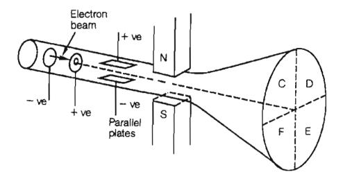
The region to which the electron beam will be deflected should both the electric and magnetic fields be operating is:
