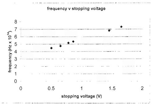
From the graph, the threshold frequency and the work function of the metal can be calculated as:
