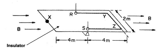
The loop of wire RYZS is mounted on an insulator as shown and is able to pivot along the line RS. All of this is then placed in a uniform magnetic field B as shown. The loop is balanced when there is no current passing through it. When a mass is placed at X a current needs to flow in the loop in order for this apparatus to remain horizontal.
