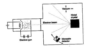
They fired electrons of known kinetic energy at a nickel crystal and used a movable detector to measure the scattering intensity at different angles.
