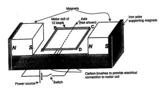
The motor coil, ABCD, has an area of  $1.70 \times 10^{-3} \text{ m}^2$  and is made from a continuous length of insulated wire wound into 12 loops. The magnitude of the magnetic field in the region of the coil is 0.22 T. When the switch is closed a current of 3.10 A begins to flow into the motor coil causing the coil to experience a torque and start to spin. When the motor coil has achieved full speed it is measured to rotate at 5.0 Hz.
