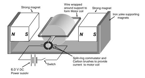
The students conducted tests on the motor and found that it operated best using a 6.0 V power supply, with the motor coil rotating at a frequency of about 3 Hz. Considering when the switch is closed the motor begins at the position shown in the diagram, explain how the torque acting on the motor coil will vary as the coil begins to rotate and reaches its full speed.
