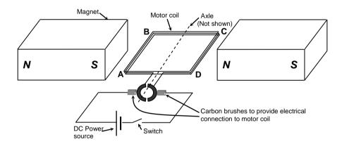
The magnets produce a field of 0.12 T in the region of the motor coil which consists of 10 square loops of 0.050 m side length. When the motor is switched on a current of 4.0 A flows into the motor coil. Which of the following alternatives correctly states the torque acting on the motor coil and the direction of the initial movement of the end of the motor coil AB?
