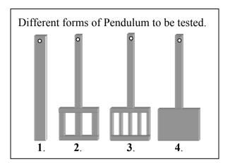
Each of the FOUR different pendulums was tested. It was observed that the motion of each pendulum was slowed as it passed between the poles of the magnet.
