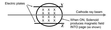
The speed of the particles in the cathode ray beam was known to be  $2.0 \times 10^5 \, \text{ms}^{-1}$ . The cathode ray beam was slightly deflected when the magnetic field was turned on. From the amount of deflection, the magnetic force on the particles in the cathode ray was determined to be  $2.2 \times 10^{-15} \, \text{N}$ .
