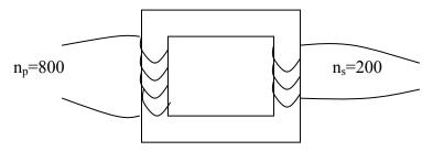
Determine the secondary current in this ideal transformer.
