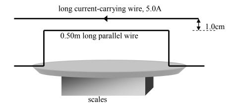
The conductors are parallel for 0.500m, and are separated by 1.0cm. A current of 5.0A is flowing through the top conductor. When a current flows through the conductor which is resting on the scales, the scales measurement *increases* by  $3.50 \times 10^{-4}$ N.
