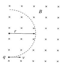
If the magnitude of the magnetic field was tripled and the velocity was doubled, what would the new radius be?
