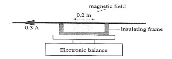
When a current of 0.3 A is passed through the rod, the reading on the balance decreases from 7.5 x  $10^{-3}$  kg to 7.5 x  $10^{-4}$  kg
