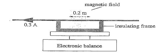
When a current of 0.3 A is passed through the rod, the reading on the balance decreases from  $7.5 \times 10^{-3}$  kg to  $7.5 \times 10^{-4}$  kg
