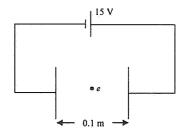
Determine the force on the electron due to the electric field.
