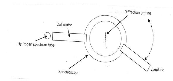
Move the eyepiece back and forth until you see the spectrum of hydrogen then make the necessary adjustments of the slit width and focus until you obtain sharp lines. Draw a diagram of what you see.
