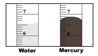
10. The diagram below shows two measuring cylinders. One contains mercury and the other water.
